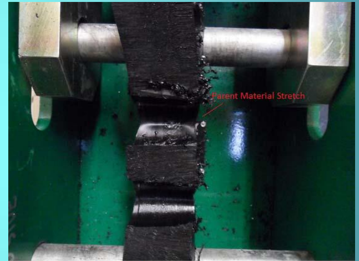
Pulling a typical pass on the tensile test
