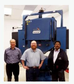
Performance Testing: 3-axis Rate Table with temperature chamber
